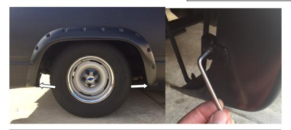
**STEP 14:** Locate the lower mounting slots in front and rear end of Fender Flare. Position the large U shape clips by sliding clips over the Fender Flare and the inner wheel arch lip so that the barb in clip inserts into the slot in Fender Flare. Apply pressure on Fender Flare to vehicle fender while tightening screws into the clips using and Allen key. Double check the front Fender Flares to make sure all screws are tight securely fastened.
