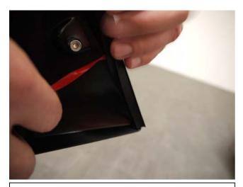
**STEP 3:** Pulling at right angles to the extrusion, remove the liner from the extrusion in small portions and apply thumb pressure to ensure that it adheres to the Fender Flares.
