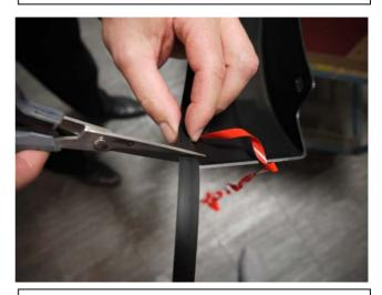
**STEP 11:** Trim any unnecessary extrusion and discard.
