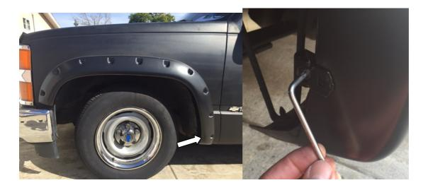
**STEP 7:** Locate the lower mounting slot in Fender Flare. Position the large U shape clip by sliding clip over the Fender Flare and the inner wheel arch lip so that the barb in clip inserts into the slot in Fender Flare. Apply pressure on Fender Flare to vehicle fender while tightening screw into the clip using and Allen key. Double check the front Fender Flares to make sure all screws are tight securely fastened.
