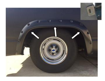
**STEP 13:** Place the Fender Flare onto the vehicle and fit into the correct position following the contours of the vehicle fender. To secure the Fender Flare to the body take the black metal clips and slide them over the Fender Flare and the inner wheel arch lip. Position the clip so that the barb in the clip locates in the slot of the Fender Flare. Install top center clip first working out to the shown locations.
