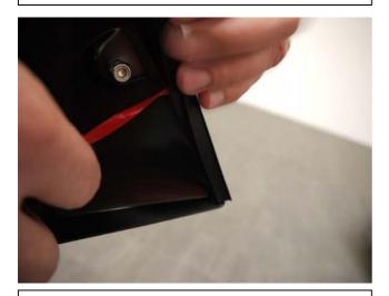
**STEP 10:** Pulling at right angles to the extrusion, remove the liner from the extrusion in small portions and apply thumb pressure to ensure that it adheres to the Fender Flares.
