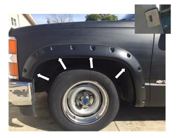
**STEP 6:** Place the Fender Flare onto the vehicle and fit into the correct position following the contours of the vehicle fender. To secure the Fender Flare to the body take the black metal clips and slide them over the Fender Flare and the inner wheel arch lip. Position the clip so that the barb in the clip locates in the slot of the Fender Flare. Install top center clip first working out to the shown locations.
